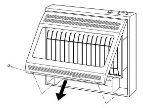
Figure 7 - Removing Front Panel Of Heater
